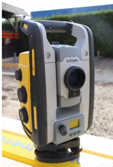
De Total station
